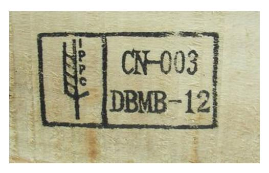
Above: Here is an example of a pallet which bears the IPPC mark. CN means that the pallet was made in China. DBMB means the wood has been debarked and treated with Methyl Bromide. Here is a pallet to avoid using for craft or DIY activities.
